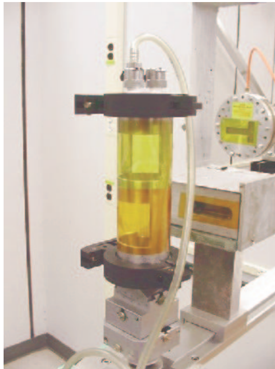
Fig.3 Helium-filled shroud with Kapton windows for the Be single crystal. The crystal will be seated in the center of the bottom window.
